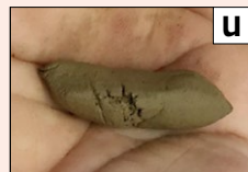
S Image 1 SAND » cannot be rolled out, gritty » sample crumbles » individual grains visible » sample grinds between teeth
